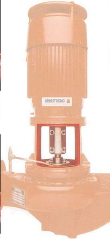
2) Remove the coupling bolts. The coupling halves (with drive and annular positioning keys) are taken from motor and pump shafts. Loosen set screws on seal rotating element and slide from pump shaft. (For inside seal see step 3)
