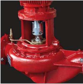
1) Split coupling with outside seal. Axially split coupling shown with coupling guard removed. Coupling bolts are still in place. Rotating element of seal is seen below the coupling, above gland plate.
